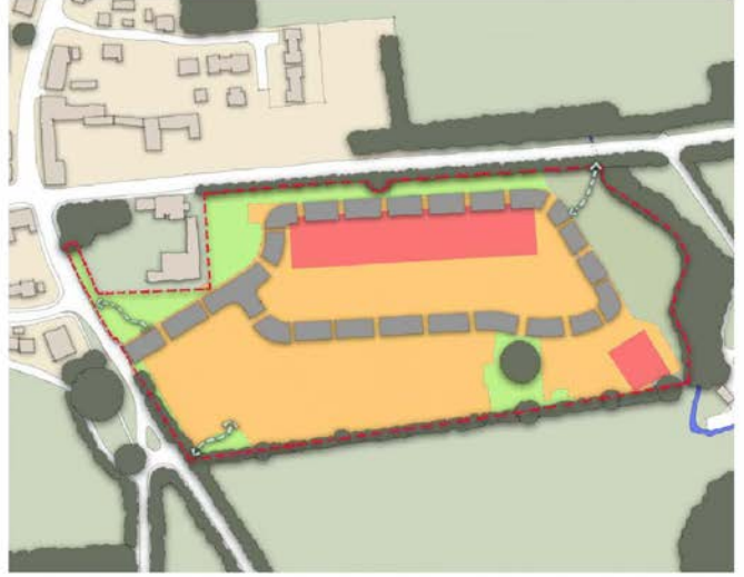
The density is at its highest at the top of the site to ensure noise levels from the A64 are minimised across the site.
